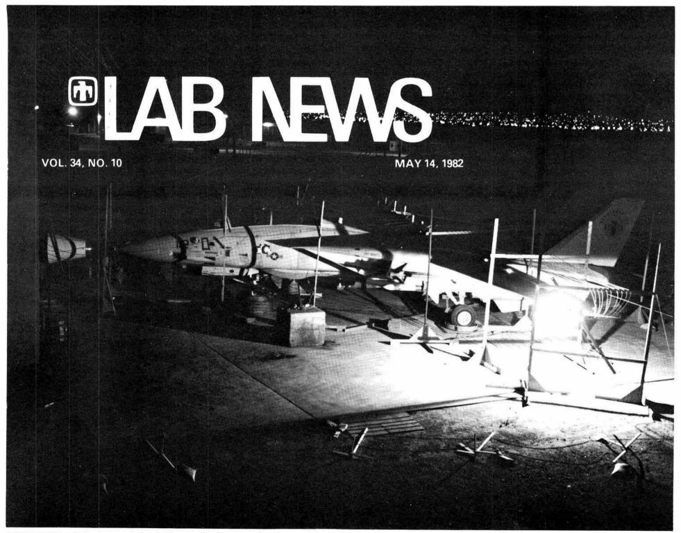
A DRAMATIC night test recently took place at the Sandia Lightning Simulator Facility during a test series performed for the Naval Air Systems Command. The Navy wanted to know how a lightning strike would affect the sensitive computer electronics on its aircraft. In the night test shown here, the F-14A aircraft (from the same squadron on the U.S.S. Nimitz that engaged the Libyan jets last year off the North African coast) was subjected to an 80,000-ampere
